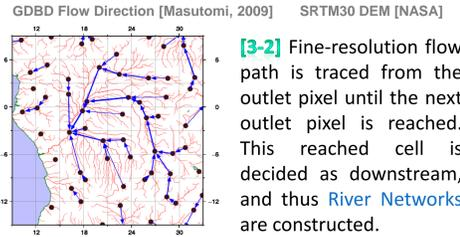
**[3-2]** Fine-resolution flow path is traced from the outlet pixel until the next outlet pixel is reached. This reached cell is decided as downstream, and thus **River Networks** are constructed.
