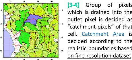
**[3-4]** Group of pixels which is drained into the outlet pixel is decided as "catchment pixels" of that cell. **Catchment Area** is decided according to the **realistic boundaries based on fine-resolution dataset**
