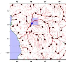
**[3-3]** **River Channel Length** is measured along with the fine-resolution flow path **considering meandering** at sub-grid scale.
