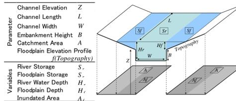
**[2-1]** River channel and floodplain storages are defined as continuative reservoirs in each grid. Total water storage in each grid is divided into river channel and floodplain storage to balance water surface elevation of both reservoirs.
