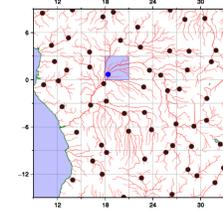
**[3-1]** A specific pixel of flow direction map is chosen as the "outlet pixel" of each coarse-resolution cell. **Channel Elevation** is decided as the elevation of the outlet pixel.
