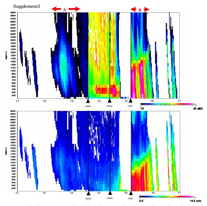
Time-height cross section of the radar reflectivity index (above) and vertical Doppler velocity (below) from 11:00 to 17:00 JST on 31 December 2004. Triangles denote the time of removing covered snow on the antenna and precipitation type on the surface. Broad red arrows on the above figure denote averaged period in the text. A and B denote the snow period and the rain period respectively.
