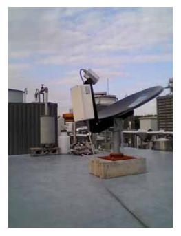
Overview of Micro Rain Radar (MRR) with a tipping bucket rain gauge behind at the roof of IIS University of Tokyo. More information is available at the Web site: http://hydro.iis.u-tokyo.ac.jp/MRR/
