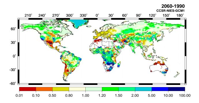
**Figure 2.** The ratio of the simulated river discharge in 2060  $(R_f)$  to that of in 1990  $(R_n)$ .
